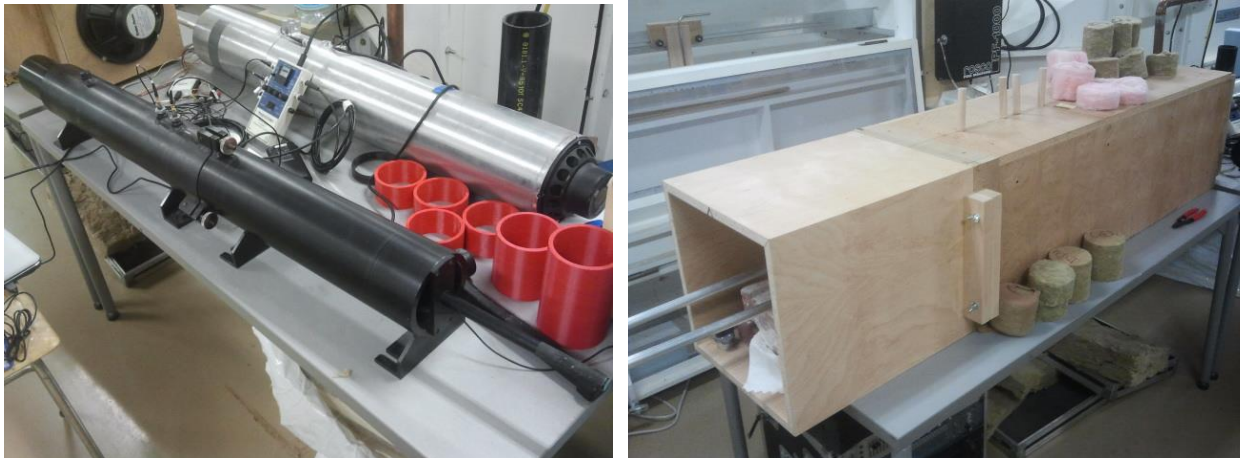
Figure 3: Circular and square impedance tubes used for the measurements.
